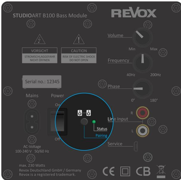
B100 Bass Module: amplifier unit rear view
