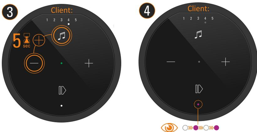
4. Wait until both devices have found each other. Then the A100 LED again shows the source with corresponding LED colour and the status LEDs on the A100 permanently show the pink LED - done.
