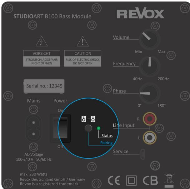
B100 Bass Module: amplifier unit rear view
