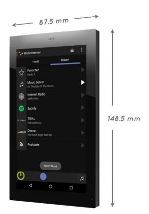
The new Revox Control Display V255 II can be used as a dedicated in-wall control for Revox Multiuser / Multiroom solutions. The Re-vox Control Display has a locked system architecture for end users so that the panel is automatically started with the Revox Multiuser App.
