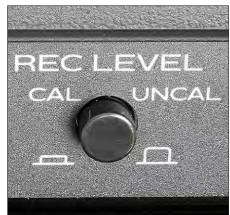
Push of a button: calibrated level via the mixing console (Cal) or recording level on the device.
