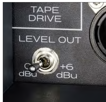
Studio or HiFi level? The output voltage can be raised by six decibels.
