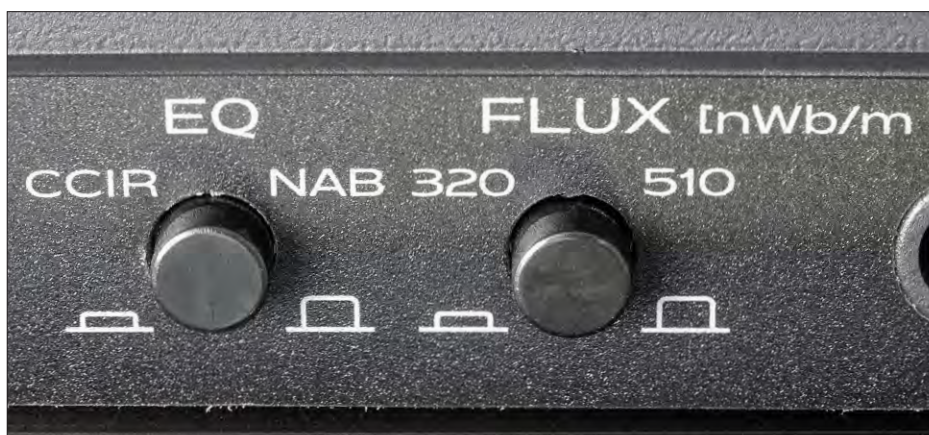
Recognizing the professional approach of the MK III: The equalization can be switched between CCIR and NAB; the magnetic flux density can be switched from 320 nanowebers per meter to 510 nWb/m.
